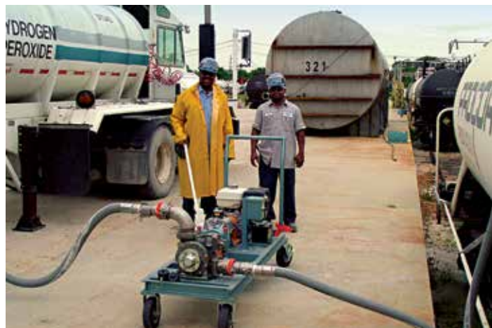
Operators at this chemical distribution/storage terminal facility transload hydrogen peroxide from a railcar to a transport via a Blackmer sliding vane pump
