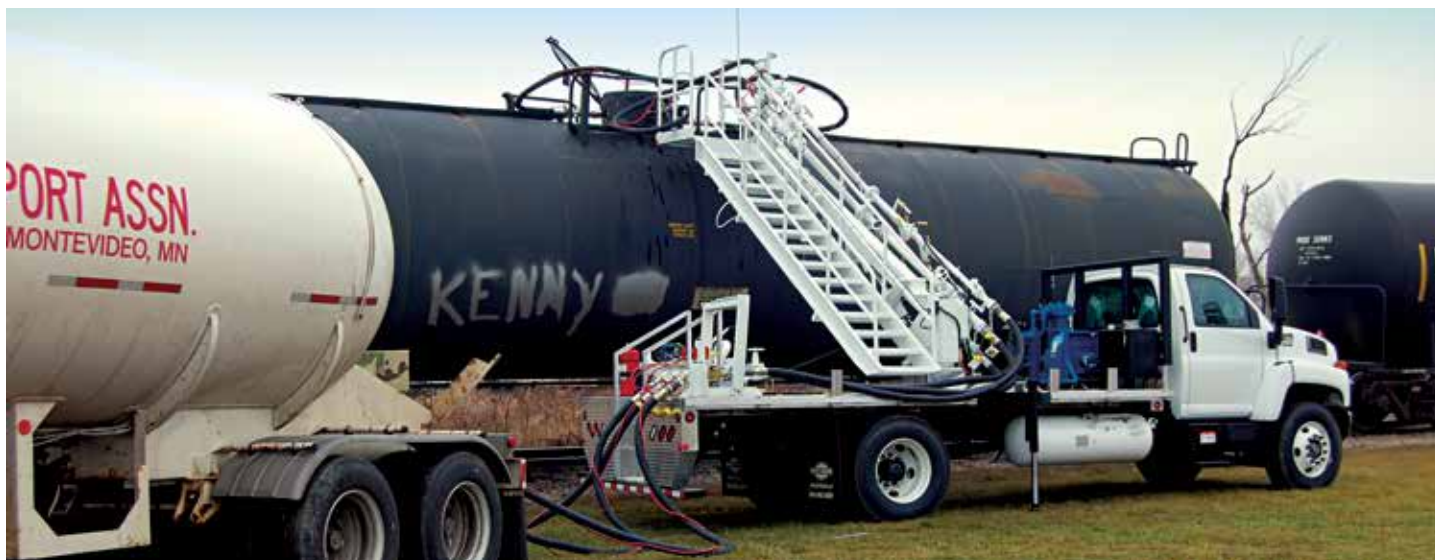
This transloading application features Blackmer compressors transferring LPG from railcars to transports
