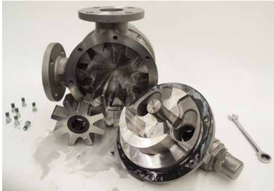
Image 3. Internal gear pumps feature a unique design that features only two moving parts, a rotor and idler gear, which allows them to operate equally well in either direction and deliver positive, non-pulsating flow of the liquid being handled.
