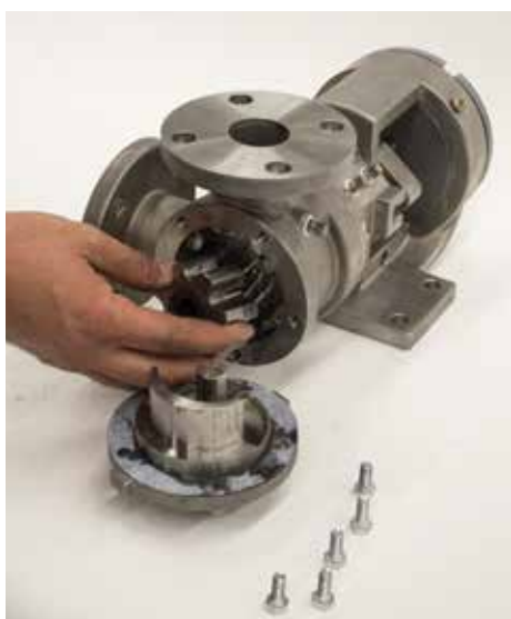
Image 4. Internal gear pumps feature a unique design that have only two moving parts, a rotor and idler gear, which allows them to operate equally well in either direction and deliver positive, non-pulsating flow of the liquid being handled.
