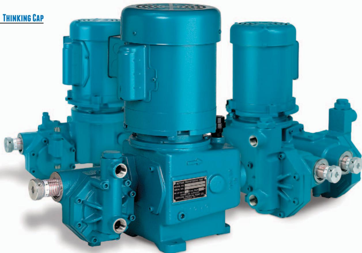
Flow rates can also be controlled automatically by a process signal and through the implementation of electric or pneumatic positioners that can adjust the stroke length, which will deliver a full 10:1 turndown ratio. In this method of control, the number of doses will remain constant with the size of each dose reduced, resulting in doses that are uniformly distributed in a constantly flowing line.
