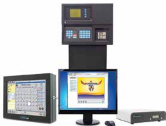
Clockwise from top: OPW's C/OPT Fuel Control System, FSC3000 Fuel Site Controller, Phoenix SQL Fuel Management Software and SiteSentinel Integra 500 Console automate, streamline and simplify inventory management and compliance documentation.
