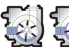
The sliding vane pumping principle is perfect for autogas handling as it delivers smooth, consistent, non-pulsating flow, even at high differential pressures.
